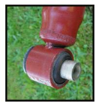
My strut just popped loose with a gentle tap from a rubber hammer, but I have read that removing the strut may be difficult because the sleeve can get stuck in the hole because of corrosion. You're on your own if you run into problems in this area.
